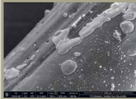
Fig. 1: Basalt integral fiber in alkaline solution after 0 days (on the left) and after 360 days (on the right) (source: ifb TU Dresden)
