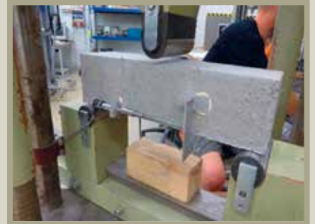
Fig. 2: Three-point-bending of a concrete bar (source: ifb TU Dresden)
